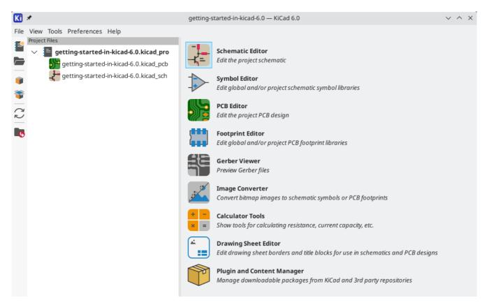
At left, the Project Files pane lists the files in the new project. There is a project file with the extension .kicad\_pro, a schematic file with the extension .kicad\_sch, and a board file with the extension .kicad\_pcb. These files all share a name with your project.
