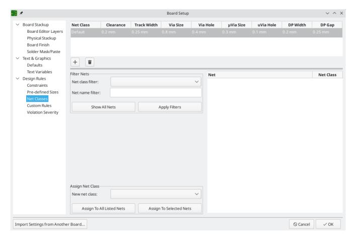
Track width and spacing can be managed manually by the designer during layout, but net classes are recommended because they provide an automatic way to manage and check design rules.
