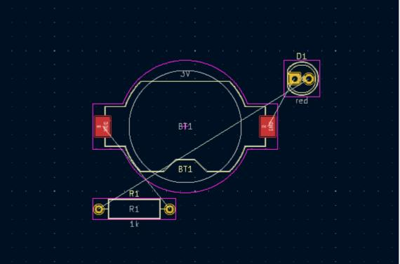
In KiCad, updating the PCB with changes in the schematic is a manual process: the designer decides when it is appropriate to update the PCB with modifications in the schematic. Each time the schematic is edited, the designer must use the **Update PCB from Schematic** tool to keep the schematic and layout in sync.
