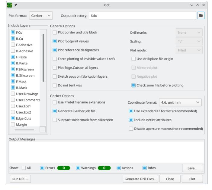
Click **Plot** to generate the Gerber files. Also click **Generate Drill Files...** and then **Generate Drill File** to create files specifying the location of all holes that will be drilled in the board. Finally, close the Plot dialog. The design is finished.
